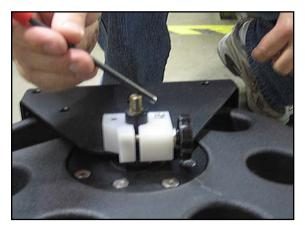
Figure 2-31. Remove Screws from Both Sides of 1st Hose Reel
