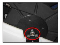
Figure 7-5. Remove Pillow Block Bearing
