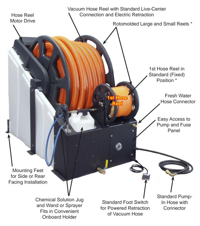
\* Small reels can be configured with solution or garden hose, all with an optional live-center connection.
