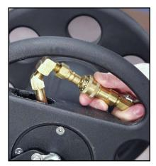
Figure 2-19. Connect Hose to 1st Hose Reel
