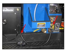
Figure 2-15. Connect Pump-in Pump Hose
