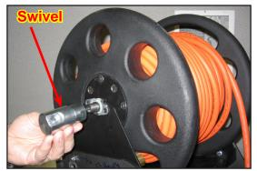
Figure 2-23. Attach Swivel onto Hose Reel
