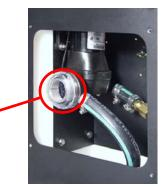
Figure 6-3. Remove Pump Access Cover
