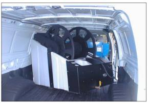
Figure 2-3. Pivot Tank over the Wheel Well
