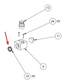
Figure 7-8. Live-Center Mount Subassembly Showing Location of 3 O-Rings (Number 10)
