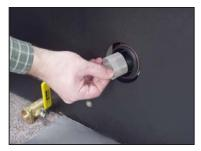
Figure 6-2. Unscrew See-through Cap (Left Photo); Remove and Inspect Filter (Right Photo)
