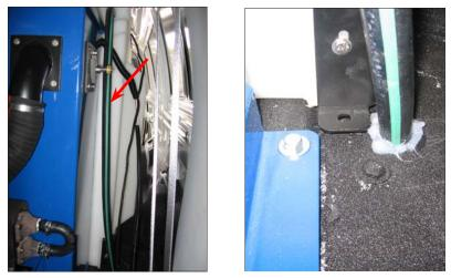
Figure 2-8. Insert Overflow Hose through Floor and Fill with Sealer
