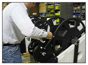
Figure 2-37. Secure 1st Hose Reel to Bracket
