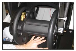
Figure 2-28. Position 2nd Hose Reel onto HydraCradle Tank
