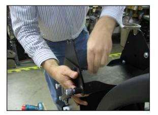
Figure 2-35. Secure Each Side of the Bracket to the Reel with 3 Screws
