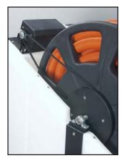
Figure 7-3. Belt Cover Removed
