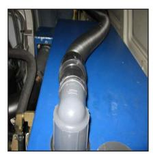
Figure 2-17. Connect Recovery Tank Hose into Cleaning Unit's Tank Cuff
