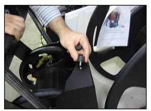
Figure 2-36. Install 2 Rubber Mounts
