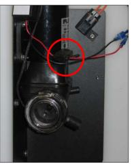
Figure 7-1. Remove 15 Amp Fuse from Fuse Holder
