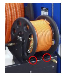
Figure 2-25. Install Clamps onto Front of Reel Bracket
