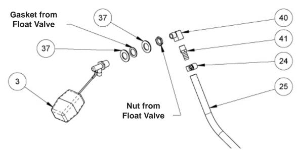
Figure 7-6. Removing Water Box Float Valve
