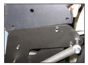
Figure 2-33. Align Holes on Bracket with Holes on Reel
