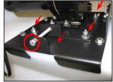
Figure 7-4. Loosen Nuts and 1 Screw on Motor Adjustment Mount
